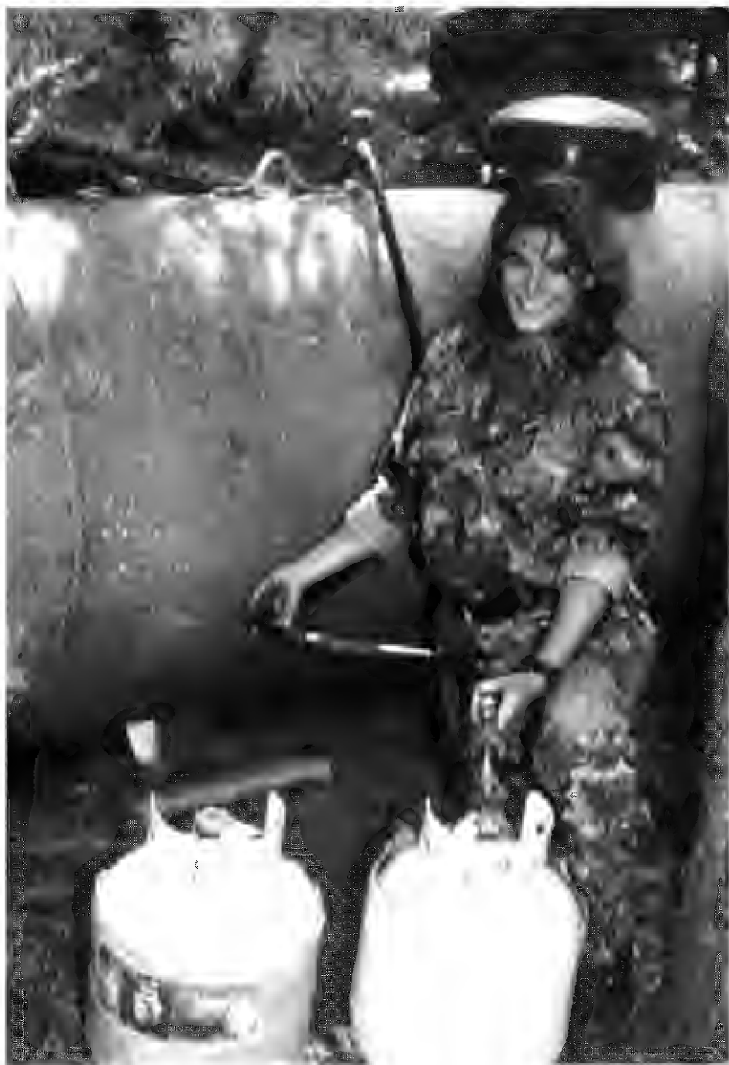
Small 5 gallon LP gas tanks can be filled from a large nurse tank if proper equipment is installed before the main tank is first filled.
