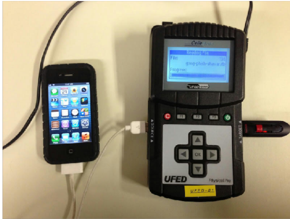
A Cellebrite Universal Forensics Extraction Device (UFED) extracting data from an iPhone 4S, 2013.
